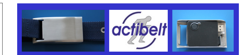
Fig. 4: The actibelt® is a belt with a high-tech buckle carrying a 3D-acceleration sensor to continuously, unobtrusively monitor long-term physical activity in the course of daily life. [1]
